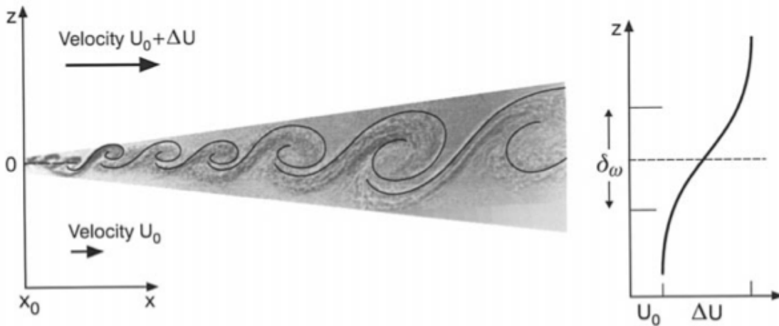
Figure 2: Instability mechanisms due to an inflected wind profile create Kelvin-Helmholtz waves. A mixing-layer develops between two coflowing air streams of higher velocity above and lower underneath. \delta_w describes the thickness of the mixing-layer [Raupach et al., 1996].
