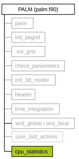
Calculate and output information about required CPU time, in total and for certain parts of PALM, e.g. "all progn. equations" or "pres" (see lecture "PALM steering")
