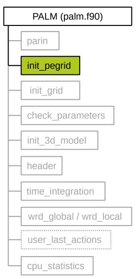
Determination of virtual processor topology (if not prescribed by user) & computation of grid point number and array bounds of local subdomains
