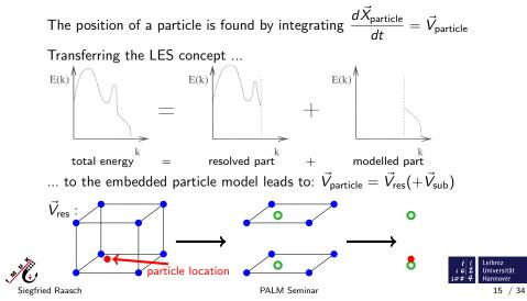
The embedded Lagrangian particle model
