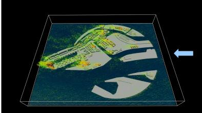
Shown is the turbulence intensity with green and red colours representing low and high values, respectively. Turbulence intensity is only shown in the area-of-interest.
